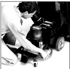
...to gain access to batteries, pad driver and all internal components.
