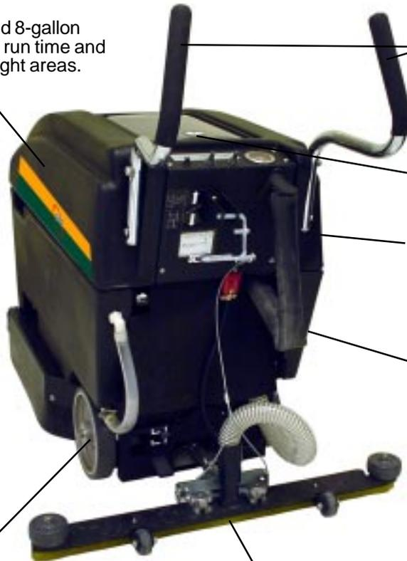
The ergonomic handles provide increased control of the machine's operation while reducing operator fatigue.
