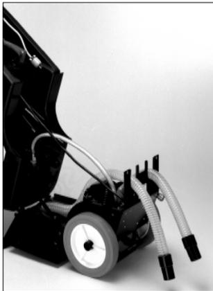
Gaining access to the internal components of the Stallion 8SC is as easy as removing two bolts and lifting up on the body.
