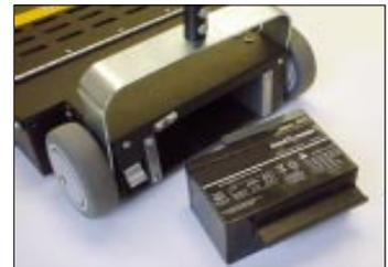
The rechargeable 12V, 9 AH battery provides 2 hours of runtime. Available extended run time battery kit provides a total of 4 hours of use.
